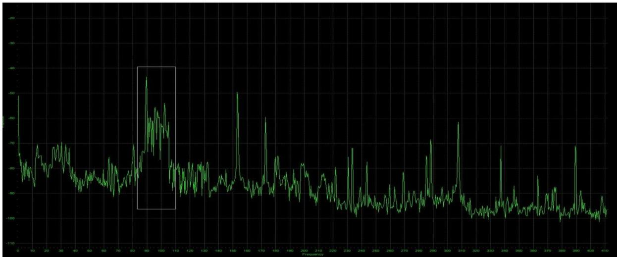
The display will adjust Frequency, span and reference level to the box you drew.
