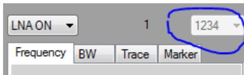
If you are running multiple SA0314 you can assign different sa0314 to different application running at the same time.
