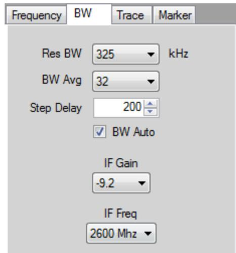
IF Frequency of the SA0314 can be changed if there is a strong signal at the IF frequency that is interfering at the current IF frequency of the SA0314.
