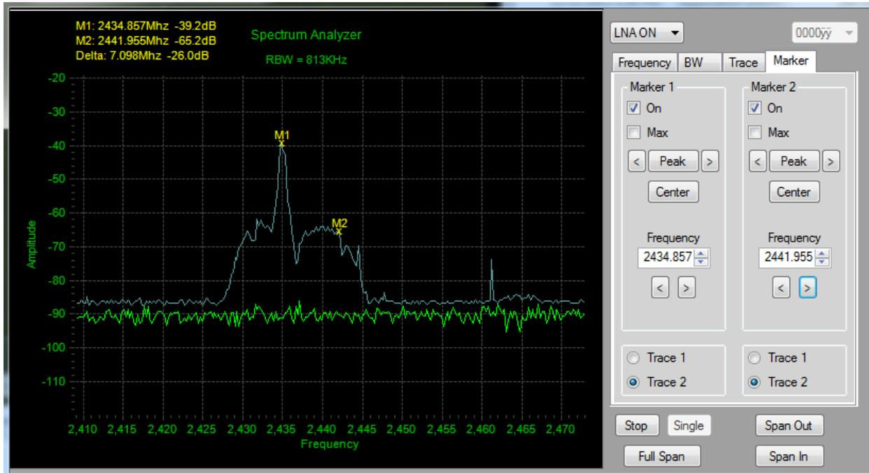
Markers are used to find amplitude at a frequency.
